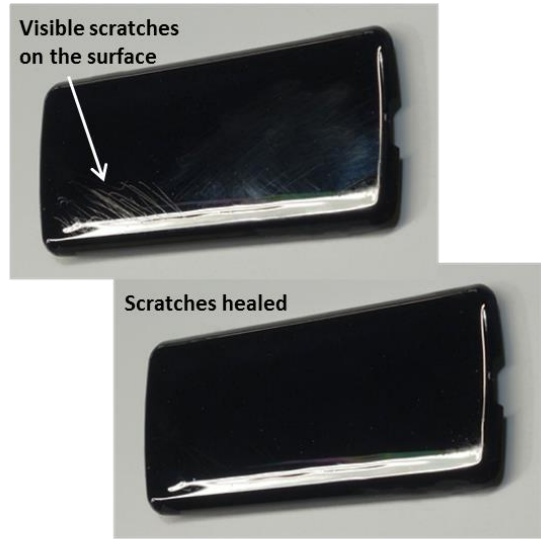
Scratches on the coatings of cellular phone covers coated with NANOMYTE® MEND exhibit healing of scratches
