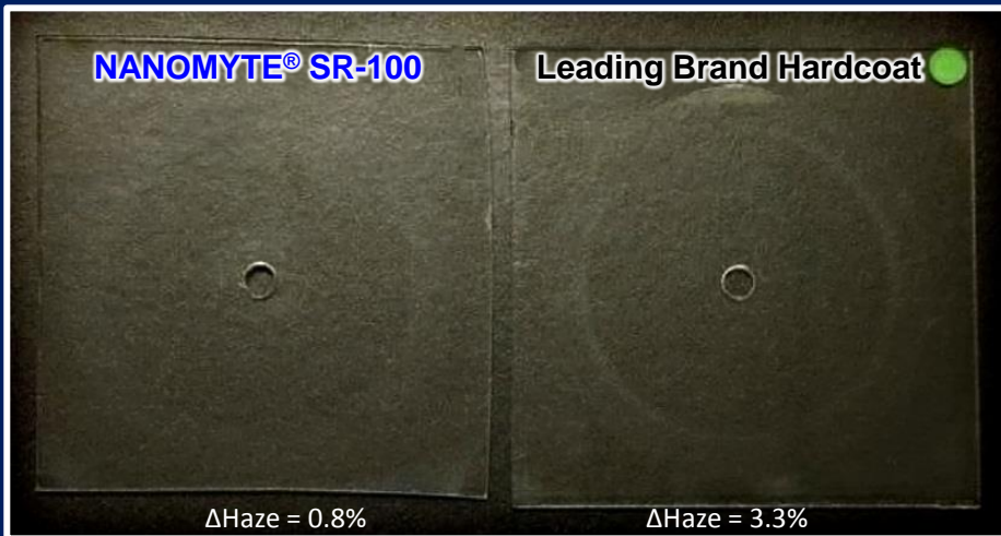
Coated polycarbonate plates after 1000 cycles of Taber abrasion testing (ASTM D-1044, 500 gram load, CS-10F wheel)
