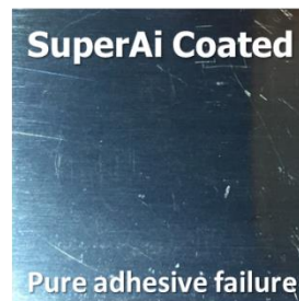
Left: Aluminum coated with NANOMYTE® SuperAi exhibits about 80% reduction in ice adhesion. Right: Uncoated surface shows cohesive failure within ice, while one coated with SuperAi had adhesive failure at the interface.
