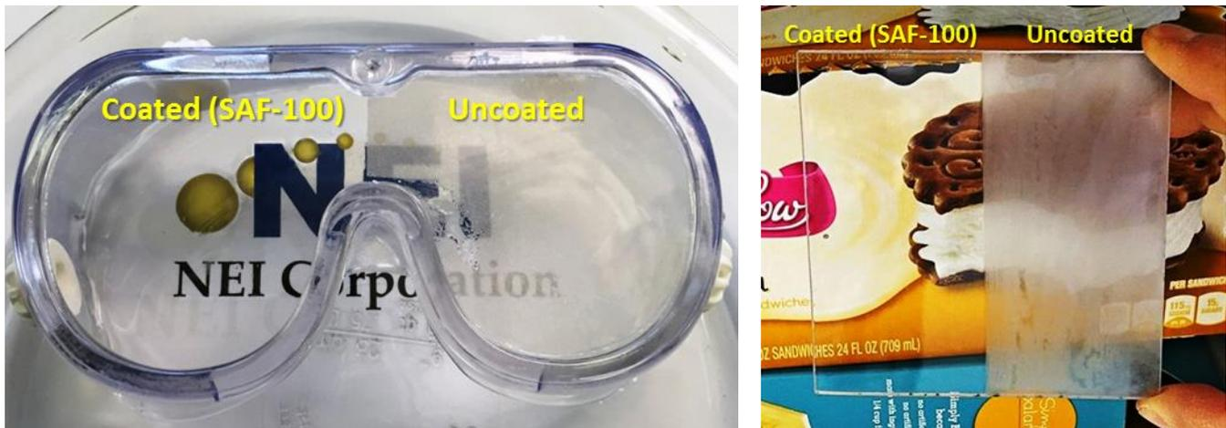
NANOMYTE® SAF-100 coated polycarbonate resists fogging over hot water (Left), and upon being removed from a freezer (right).
