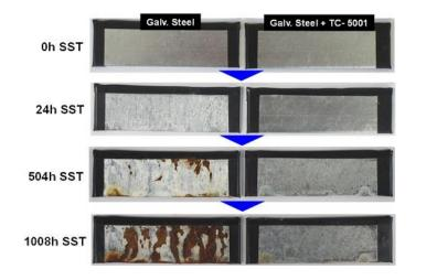
Clear TC – 5001 coating on galvanized steel provides significant corrosion protection: no red rust even after 1000 continuous hours of Salt Spray Testing (ASTM B117)
