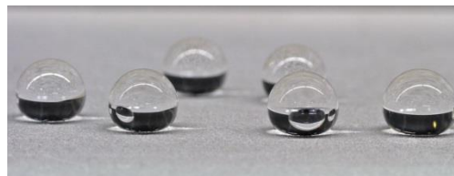
Liquids easily roll off surfaces treated with NANOMYTE® SuperCN Plus, forming droplets with contact angles as high as 165°.
