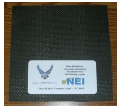
Figure 2: (Left) – Schematic of a core-sheath fiber showing the straw-like morphology; (Right) – FRC coupon containing self-healing, core-sheath fibers.
